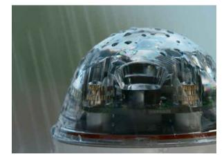
Our sensors can be set to automatically open and close the roof depending on the weather conditions. Re-opens to the last known position or any pre-set position programmed.
